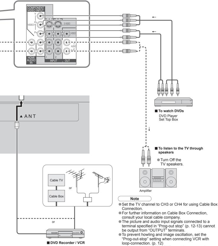
• When equipment (STB, DVD, etc.) is connected to HDMI or COMPONENT terminals, only audio signals can be obtained. No video signals can be output.
